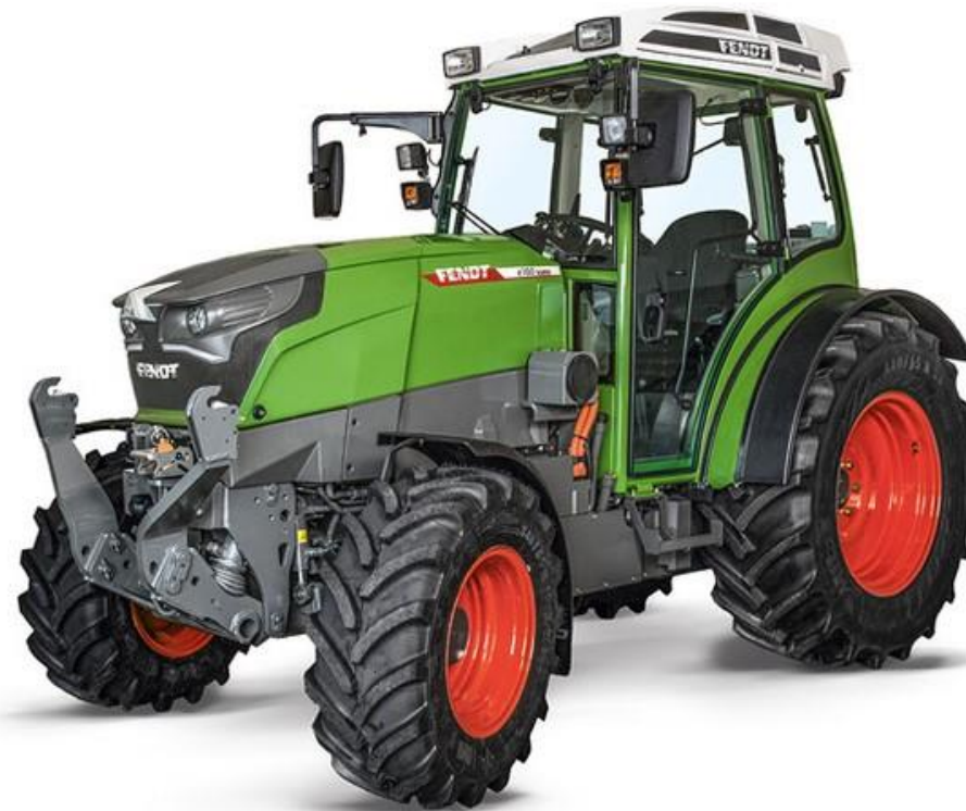
Fendt e100 Vario electric tractor (50kW / 75hp) 100 kWh battery – V2G (vehicle-to-grid) ready Extended field trials 2019/20 in Germany
