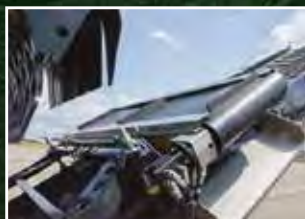
MAGNETIC SEPARATOR FOR EXTRACTION OF FERROMAGNETIC MATERIALS.
