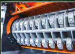
SHREDDING SHAFT EQUIPPED WITH 36 KNIVES, TO WORK WITH PALLETS, GREEN AND WOOD WASTE
